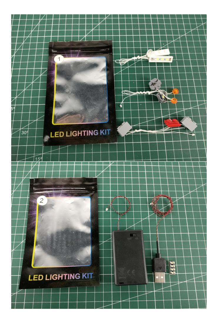
Take out the USB power cord and a 4-seat expansion board, and then tear off the seal of the expansion board. Coming with usb cable and battery box for choose, can be powered by power bank/wall charger or you can also use it with the battery.
