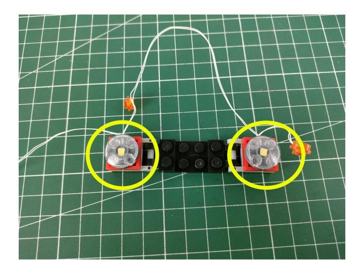
Put the yellow lighting parts through the small holes in the picture, and then place the lighting lines in the gaps between the building blocks.
