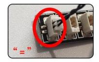
Connect the USB power cord and expansion board together.
