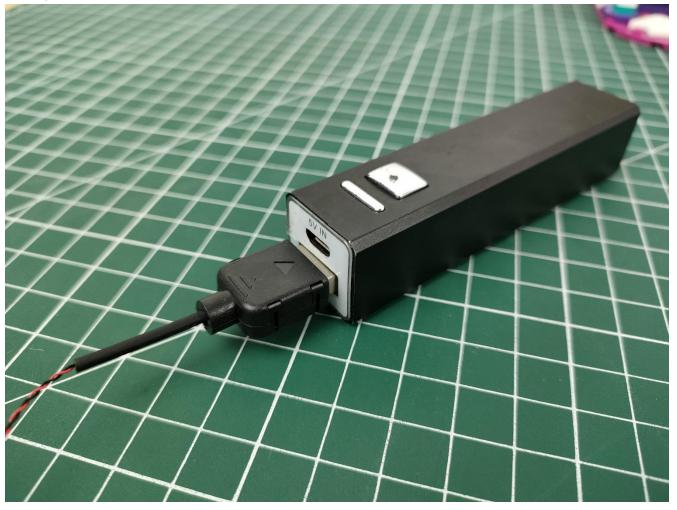
Connect the USB power cord to the RGB remote control module.
