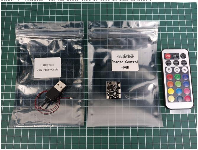
The power supplies that can be used with the USB power cord are as follows (the voltage for normal use is 5V).
