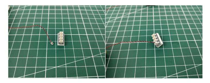
Connect all the component in No.1 bag and No.2 bag to the Expansion Board in same way just as shown.
