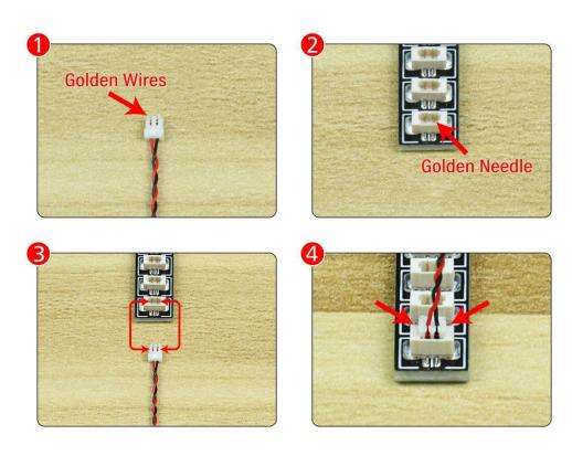
Connect the Expansion Board and AAA Battery Box as shown.
