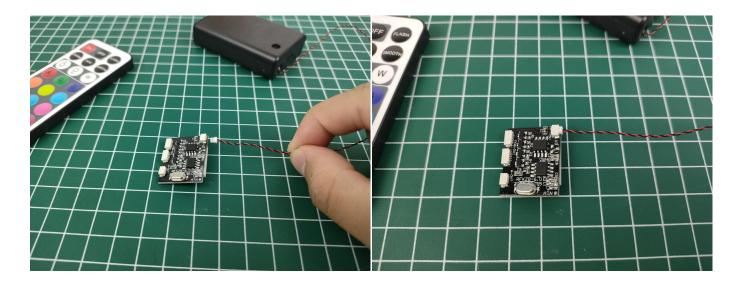
Connect all the components in No.1 bag and No.2 bag to the RGB Remote Control Board in same way just as shown.
