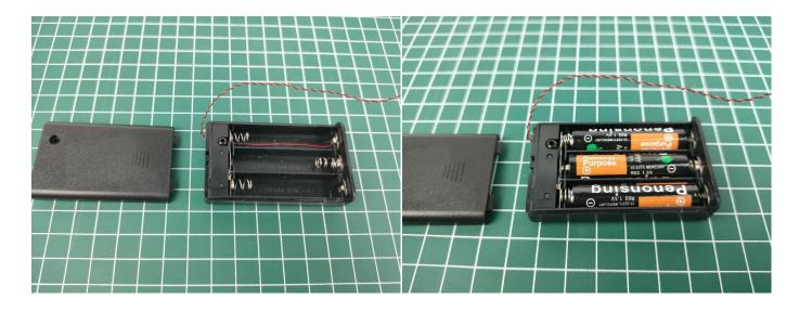
Connect the RGB Remote Control Board and AAA Battery Box as shown.
