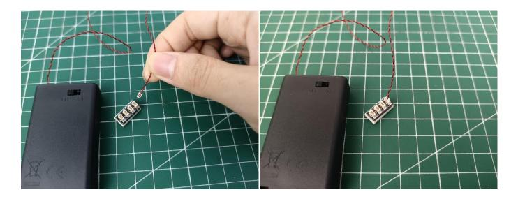
Connect all the components in No.1 bag to the expansion board in same way just as shown. Turn on the battery box, all the lights are on as shown.
