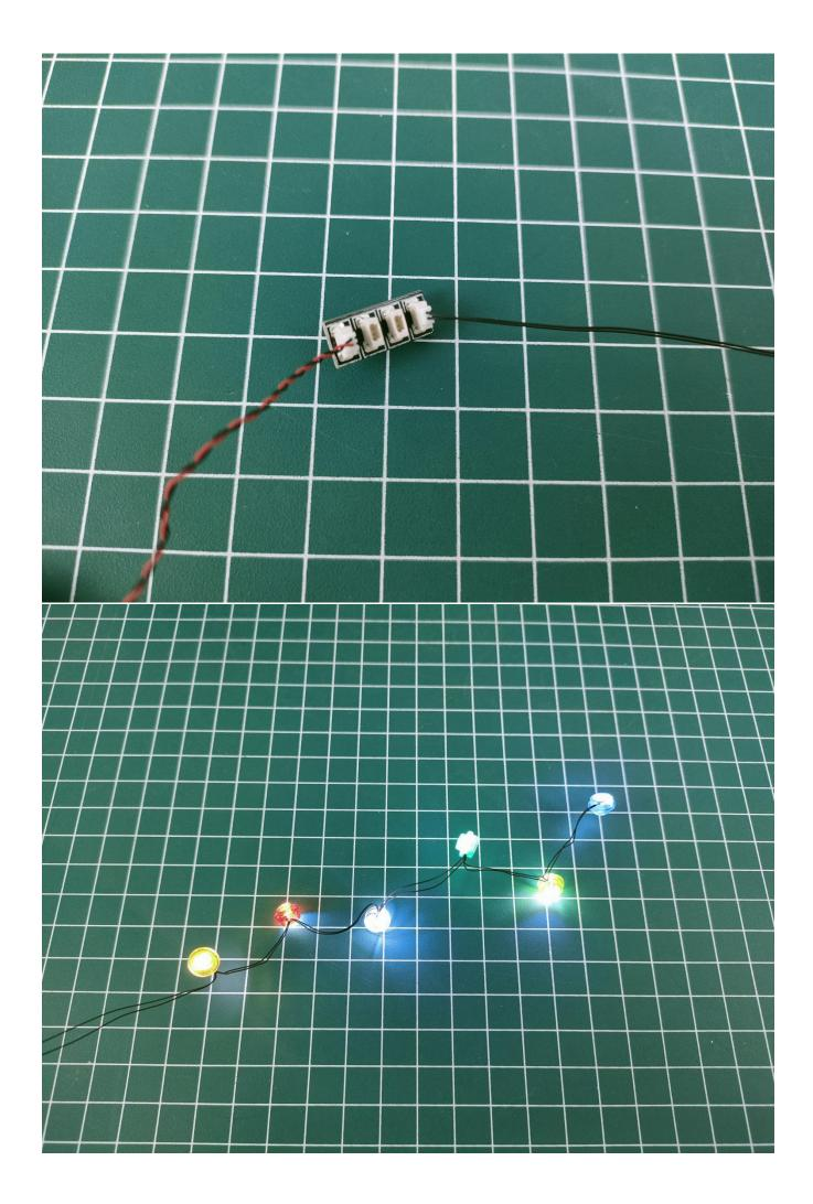
After the test is complete, unplug the lighting from the expansion board. Put the non-abnormal lighting parts back into the original bag first.
