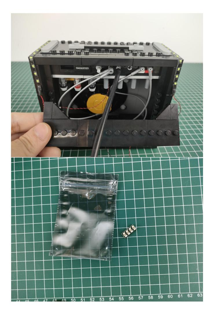
The two lighting wires inside are connected to the 4-seater expansion board.
