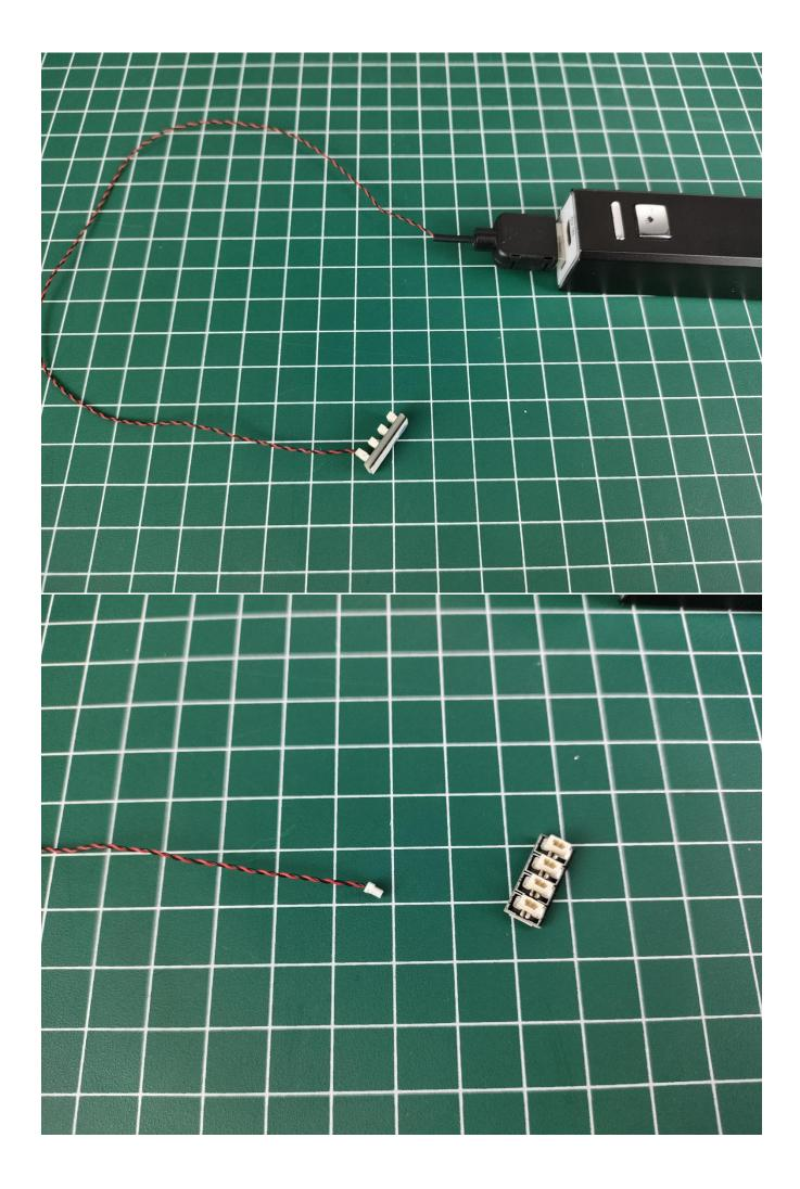
The light strip wires on both sides are connected to the 4 expansion boards.
