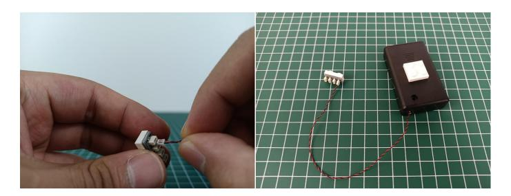
Connect all the components in No.1 bag, No.2 bag to the Expansion Board in same way just as shown and turn on the battery box, all the lights are on as shown.
