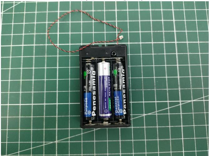
Install 3 AAA batteries (note the positive and negative poles).
