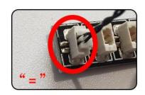
Connect the expansion board and the battery box.
