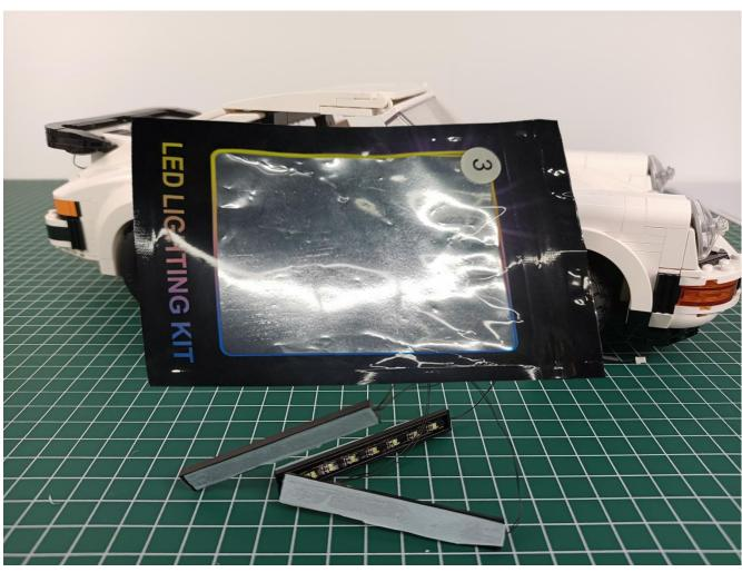
All lightings are connected to the remote control switch module, pay attention to the direction of the terminal.
