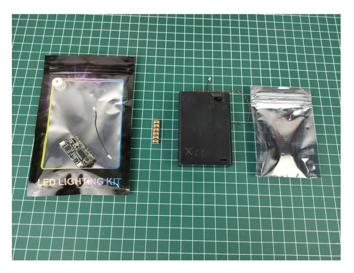
Then take out the USB power cord and an expansion board from the small bag. The usage of the USB power cord is similar to that of a battery box, and it can be powered by a power bank or a mobile phone charger. The battery box and the USB power cord can be freely chosen, choose one of the two (the USB power cord is used in this article).
