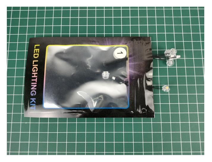
In order to avoid not lighting up after installation, the lighting in other bags should be tested in the same way before installation.
