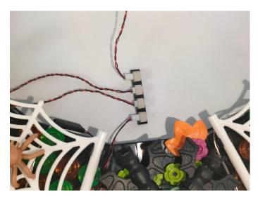
27. Peel off the adhesive paper on the expansion board and stick it onto the inner wall of the garland.
