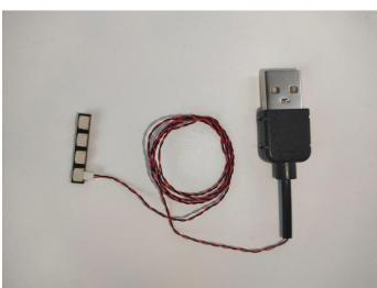
26. Connect the lamp wire to the expansion board.
