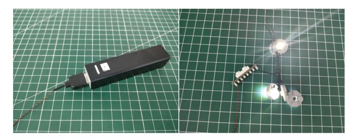
Unplug this components and put it back in the corresponding bag. There are one in bag NO.2, two in bag NO.3, two in bag NO.4 need to be tested.
