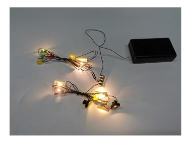
Unplug these two components and put them back in the corresponding bags. Attention that after the test is completed, each components should put back in the corresponding bag including the socket and the battery box.
