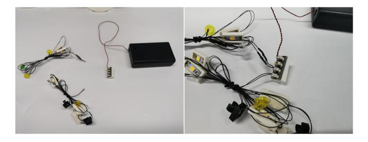
Turn on the Battery Box, all the lights are on as shown.
