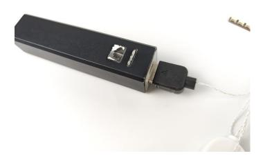
When we test the "①" light strip, please remove one of the strips and connect it to the socket. Turn on the portable power bank, and the lights will illuminate normally, as shown in the following image.
