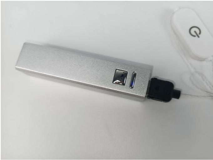
When we test the "①" light strip, please remove one of the strips and connect it to the socket. Turn on the portable power bank, and the lights will illuminate normally, as shown in the following image.
