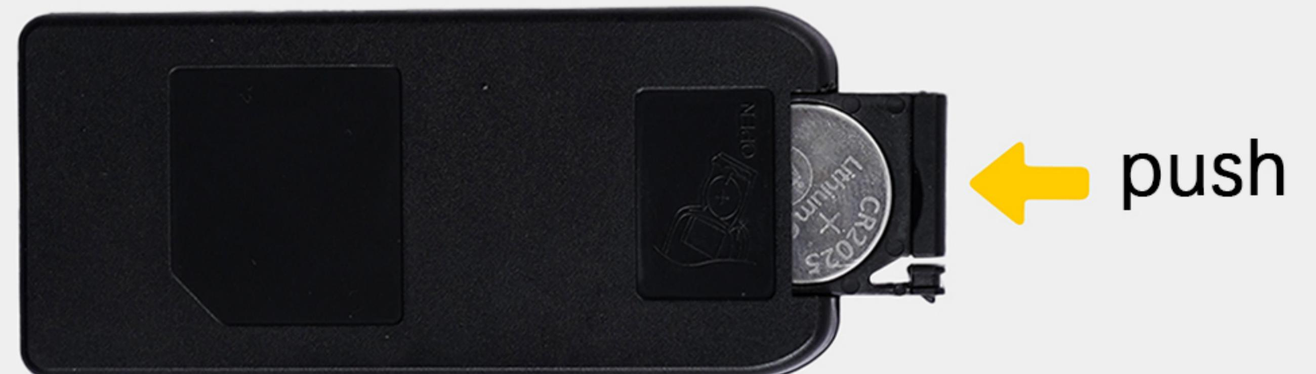
**Note:** This product is equipped with a child lock. To open the battery compartment, first press the switch inward, then pull outward at the same time.
