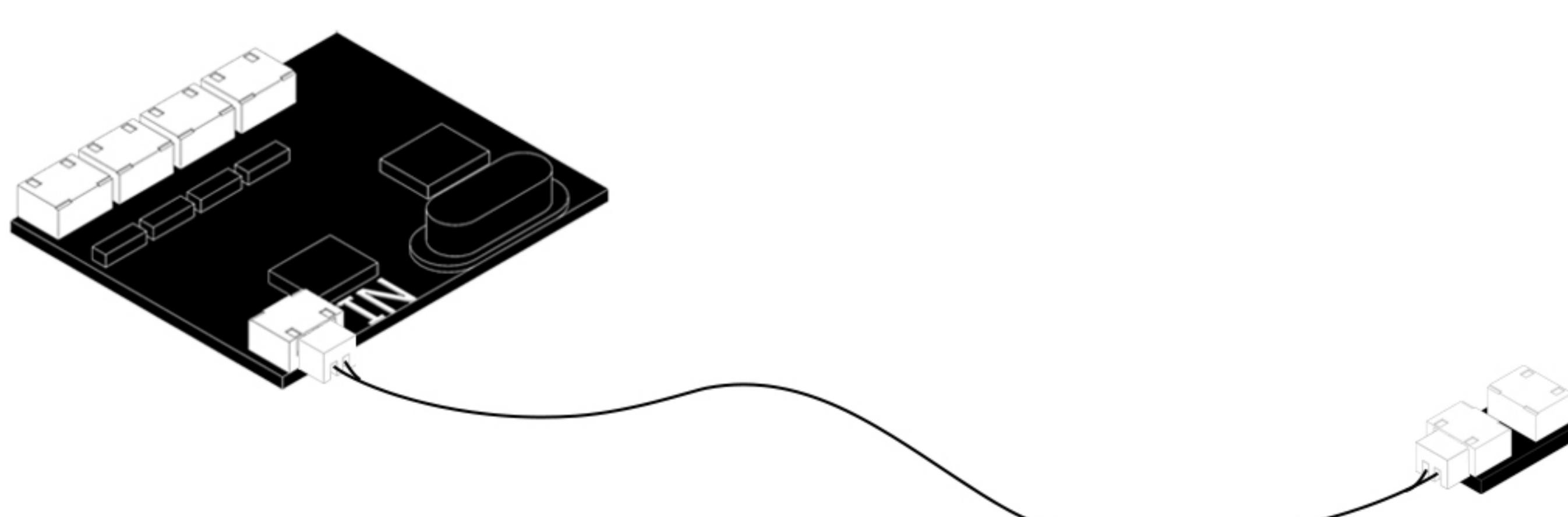
EN:19. Take out the power cord from bag A01305 and connect it to the expansion board.
