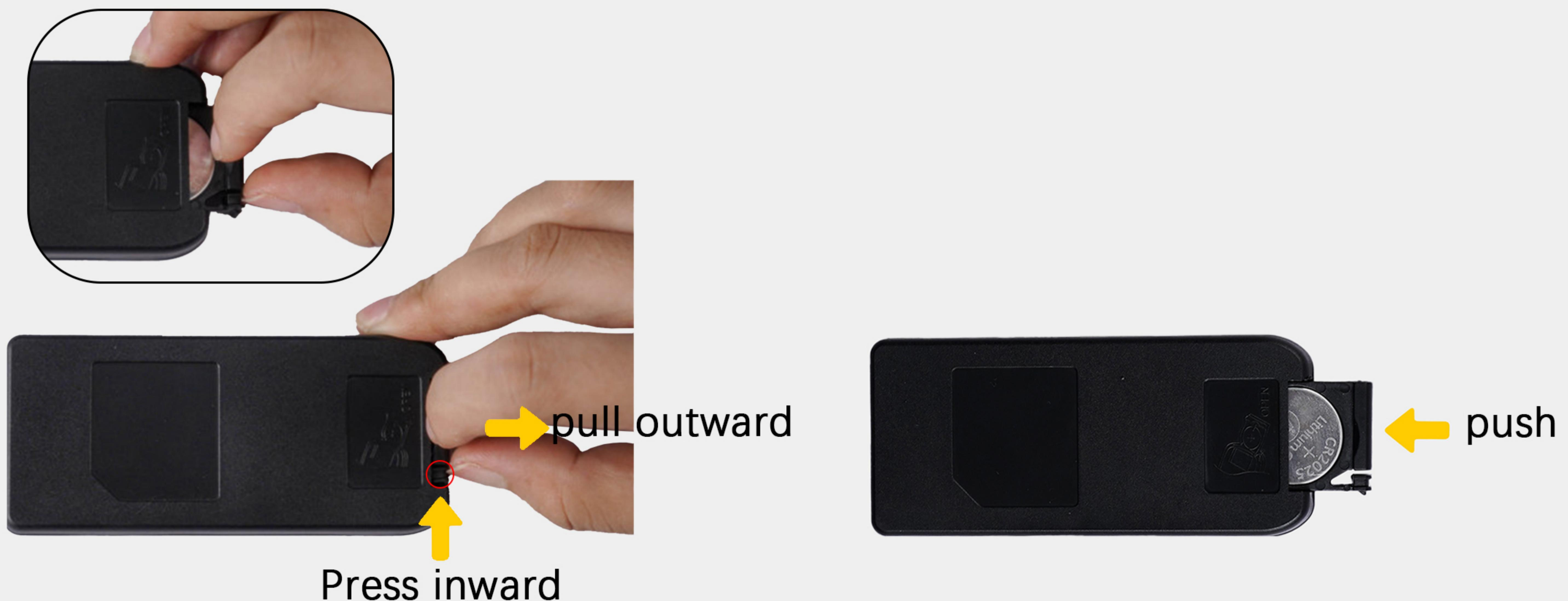
**Note:** This product is equipped with a child lock. To open the battery compartment, first press the switch inward, then pull outward at the same time.
