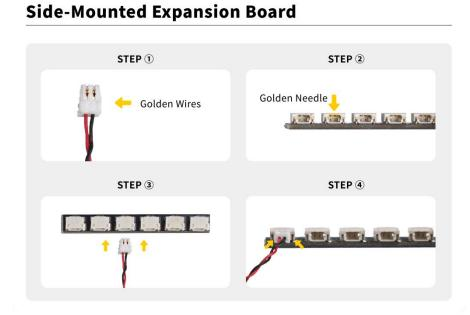
All our connections between plug and socket are all the same as shown above. So for any such structure with plug and socket, please pay attention to the golden wire of the plug and the golden needle of the socket, they must be touched together.
