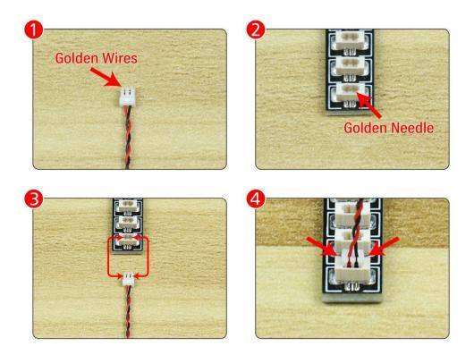
Connect the Expansion Board and AA Battery Box as shown.
