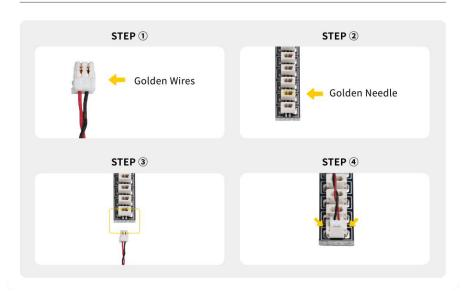
The connection method between the touch dimming module and expansion boards is as follows:
