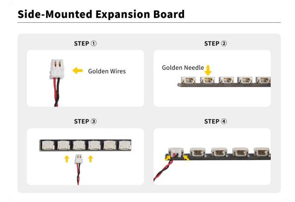
Connect the Expansion Board and USB Power Cable as shown.
