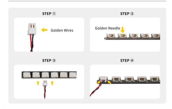
Connect the Expansion Board and USB Power Cable as shown.
