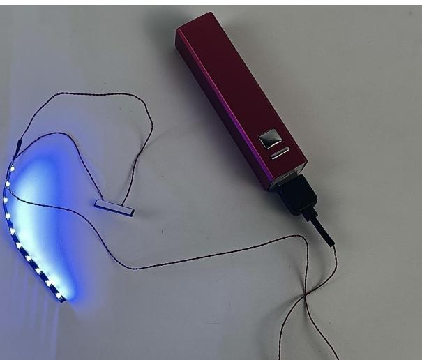
Test each lamp according to this method. It should be noted that after the test, the lamp must be returned to the corresponding bag to avoid confusion of types.
