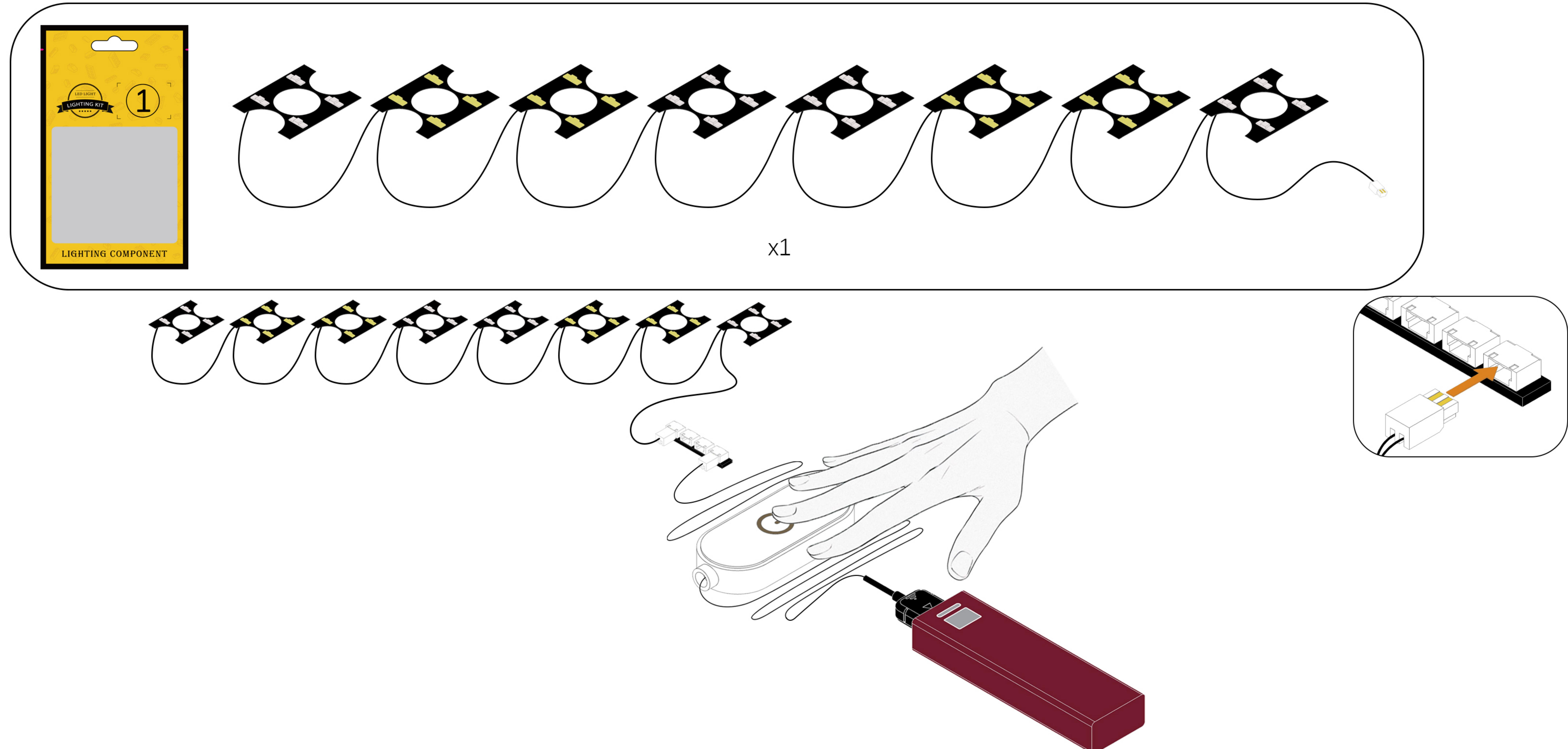
After confirming no abnormalities, temporarily return the light string and expansion board to their original bag, then proceed to test the lighting fixture.
