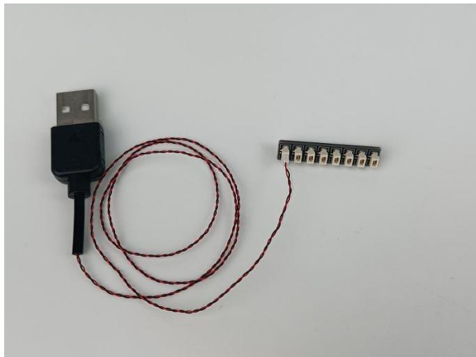
The usb power cable can be powered by phone chargers, power banks,etc.
