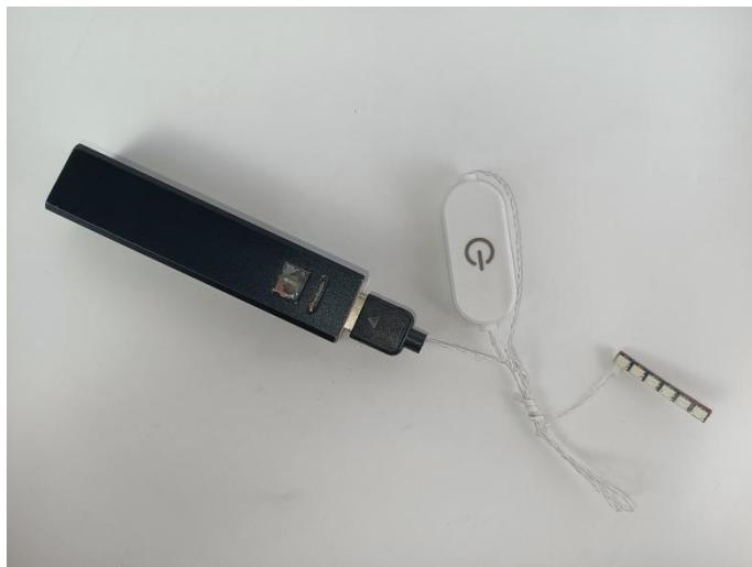
When we test the "③" light strip, please remove one of the strips and connect it to the socket. Turn on the portable power bank, and the lights will illuminate normally, as shown in the following image.
