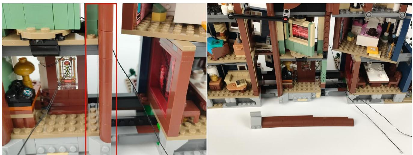
53. Use a pry tool to pry open the building block, then route the lamp wire around the protruding points of the building block, and finally press down on the building block.
