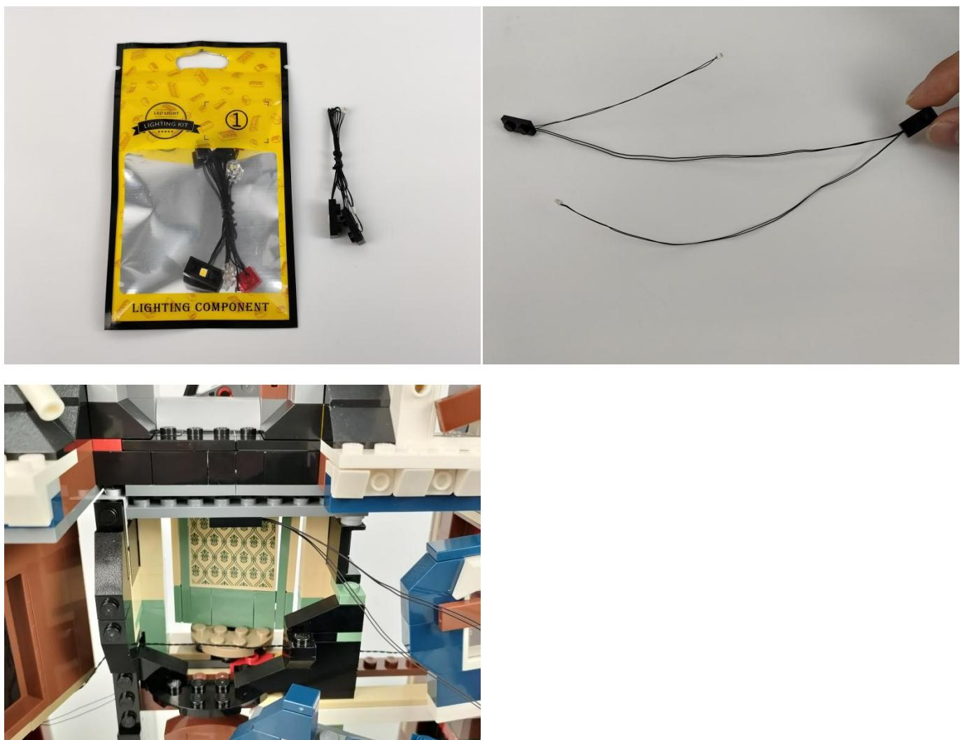
65. Pulling the building block components on both sides will make the building block door rotate.
