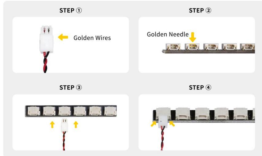
All our connections between plug and socket are all the same as shown above. So for any such structure with plug and socket, please pay attention to the golden wire of the plug and the golden needle of the socket, they must be touched together.
